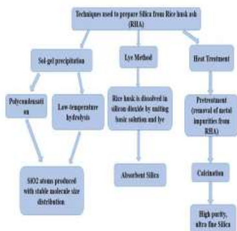
Figure 2: Illustrates the methods to produce silica using the ash of rice husks (RHA)
