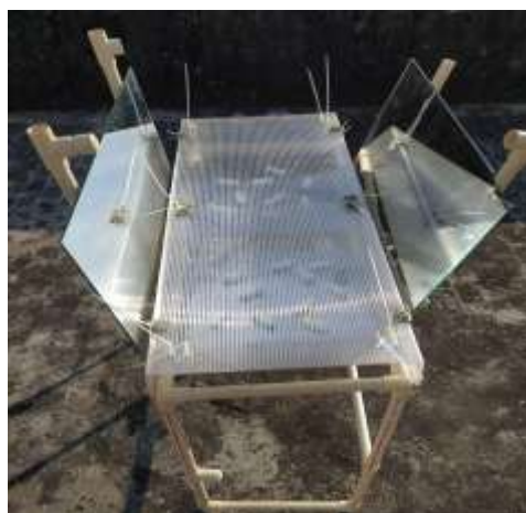
Fig. 1. Photographic image showing coconut samples placed in stainless steel and aluminium absorber plate in the solar dryer setup.
