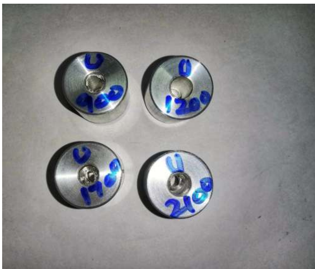
Fig. 4. Samples drilled using Uncoated drill.
