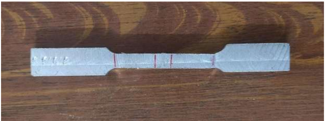
Fig. 5. Tensile test Dogbone sample
