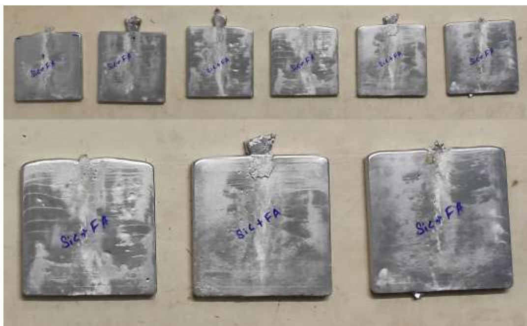
Fig. 3. Experimental Group(Al6061+SiC+Fly ash) Sample
