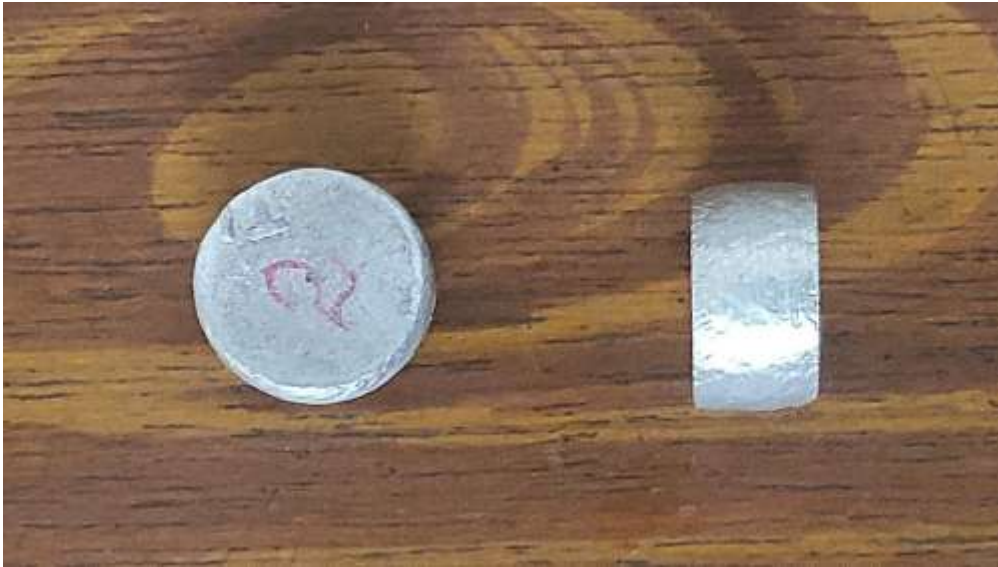
Fig. 6. Compressive test cylindrical sample
