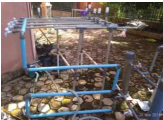
Figure 5 The unit for reducing Fe levels consisting of artificial venturi, buffle, temporary deposition and filtering is seen from the left side
