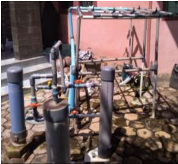
Figure 3 Fe level reduction unit consisting of factory venturi, buffle, temporary deposition and filtering viewed from the front.
