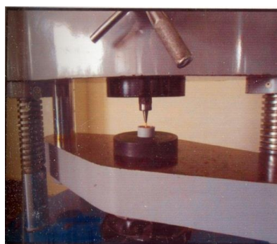
Fig. 4: Sample in placed in Universal Testing Machine
