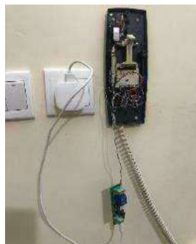
Fig. 24: Connecting SSR to power
