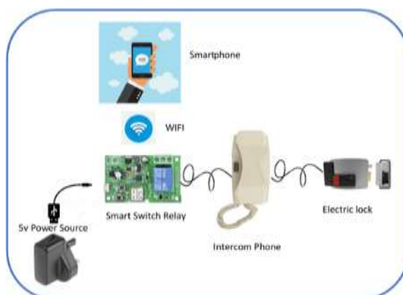
Fig. 13: block diagram of the automated door system
