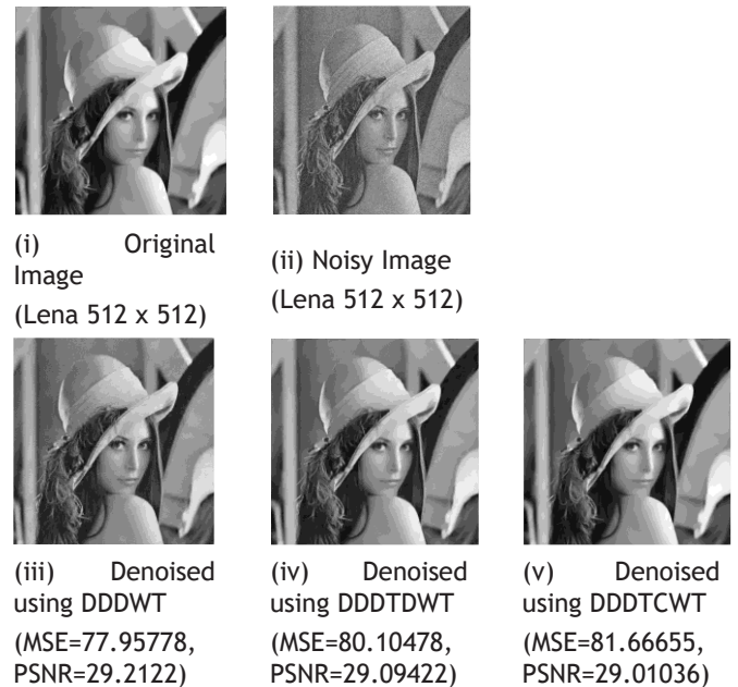
Fig. 7(a). Represents (i) Original Image, (ii) the noisy image and (iii) to (v) denoised images obtained using DDWT, DDDTDWT and DDTCWT techniques respectively with ( \sigma = 20 ) for Lena 512 x 512 image.
