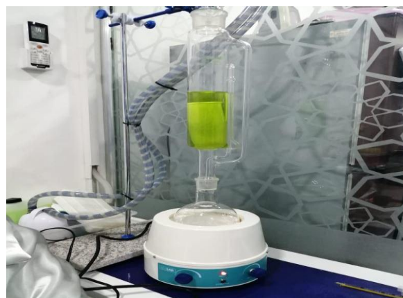
Figure 2 : Tribulus terrestris T plant extract in Soxhlet
