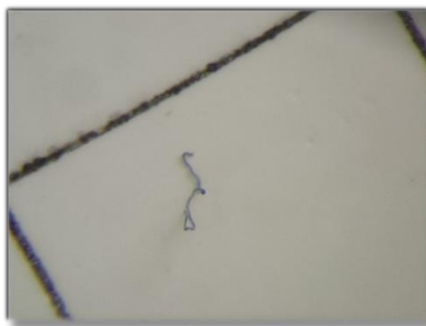
Fig (6) Microplastic particles on the surface of the filter sheet
