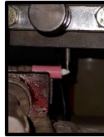
Fig 5: Tooth placed in Universal testing machine
