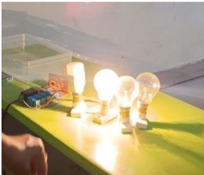
Fig. 2: Lights turned on in accordance with user's eyeblinks
